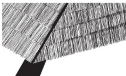
4. Continue up the roofline cutting strip and nailing until the entire structure is covered.
