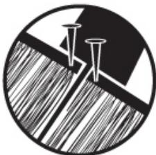
3. Thatch strips are cut in the middle of the corner rafters and secured by nails. Step 5 will cover any gaps.
