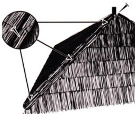
5. Place the tapered end of the corner hip at the top with the batten facing underneath. Nail to the corner rafter - bottom, top and in the middle.
